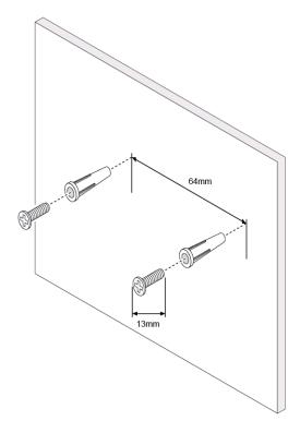
STEP 2 Maneuver the Switch to insert the screws into the two slots, then slide the switch downward onto the screws.
